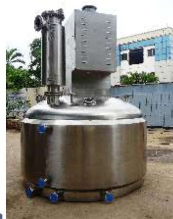
Above: CE lid design with Single Piece vessel-bottom supply option
