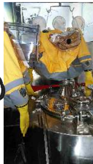
Left: ANFD with Integral Barrier Isolator (Glove box)
