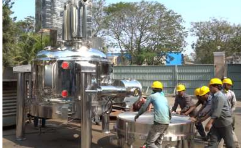
Above: CE lid design with Dual Piece vessel-bottom (detachable on wheels)
